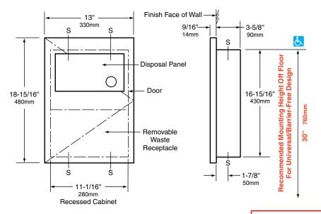
Rough Wall Opening 11-1/2" (290mm) wide 17-1/4" (440mm) high 3-3/4" (95mm) minimum recessed depth
