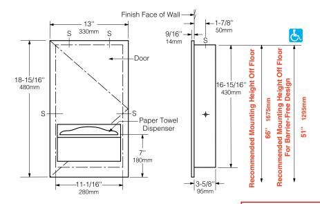
Rough Wall Opening 11-1/2" (290mm) wide 17-1/4" (440mm) high 3-3/4" (95mm) minimum recessed depth
