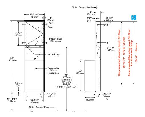
Rough Wall Opening 16" (406mm) wide 54-3/4" (1390mm) high 4-1/4" (108mm) minimum recessed depth
