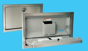
**KB110-SSRE HORIZONTAL, RECESSED-MOUNTED** Dimensions: 37"W x 23"H (940 x 584 mm) • Depth (closed): ¼" (6 mm) • Extension (open): 15" (381 mm) • Rough Wall Opening: 35½" W x 20½" H (900 x 529 mm) • Depth: 4¼" min. (108 mm)
