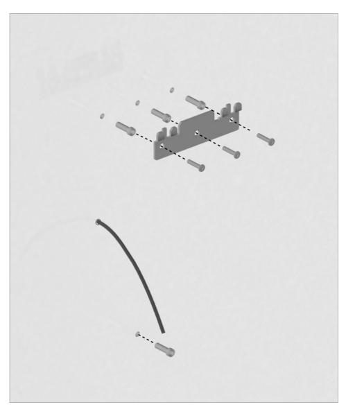
Once the marks have been made, attach the wall bracket to the wall and prepare the cable to the electricity network.
