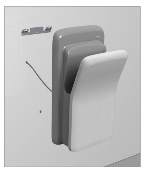
Place the ffuuss<sup>™</sup> handryer2 on the wall bracket, remove the air intake filter and fix the unit via the inner hole. Insert the filter and connect the unit.
