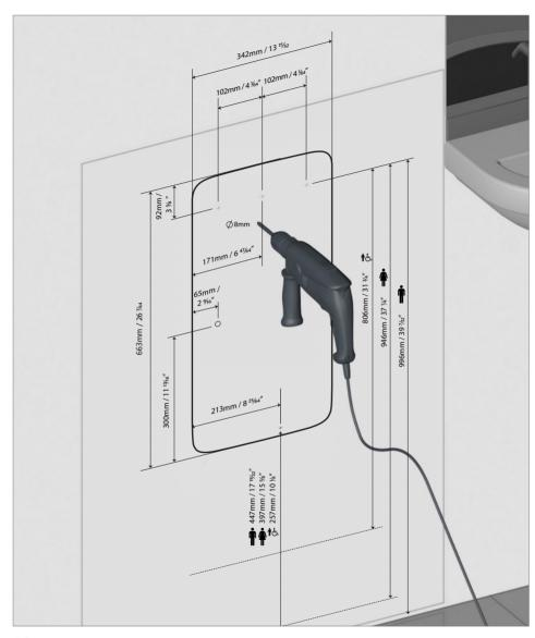
Place the ffuuss™ handryer2 template against the wall where it will be installed and make the holes according to the diagram. Check beforehand if there is a direct cable to the electricity network or if it has to be connected using a plug.
